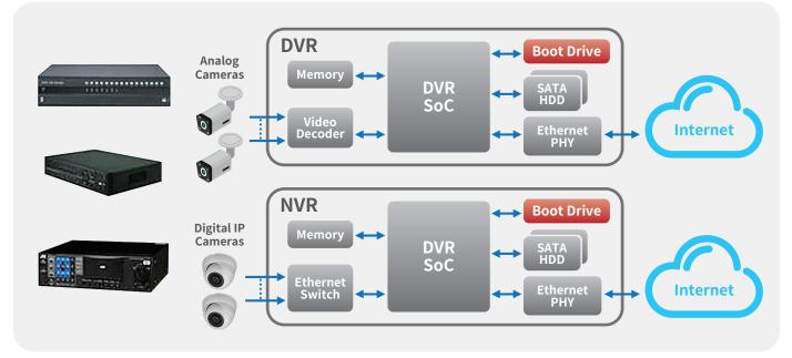
Figure 2: Ferri series boot disks for monitoring equipment such as DVR, NVR and IP Camera.
