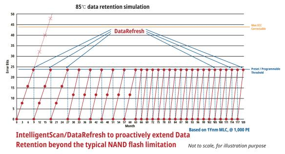
Figure 5. IntelligentScan ensures reliable data retention for the lifetime of the storage device.
