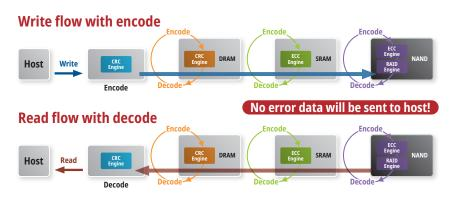
Figure 3: End-to-end data path protection ensures data integrity in Ferri storage
