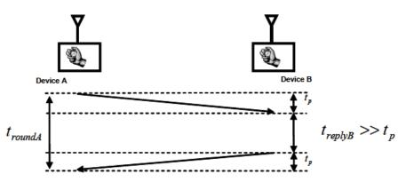
Figure D1.5—Exchange of message in two-way ranging
