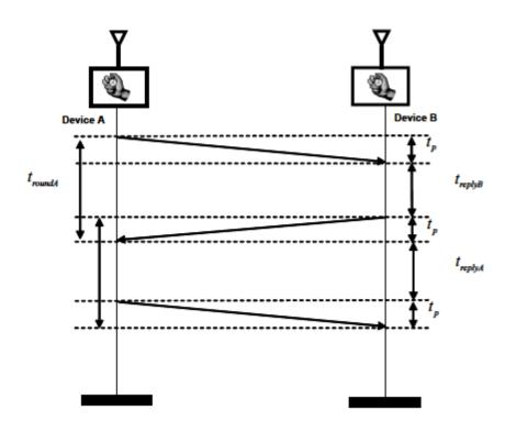
Figure D1.6—Exchange of message in SDS-TWR
